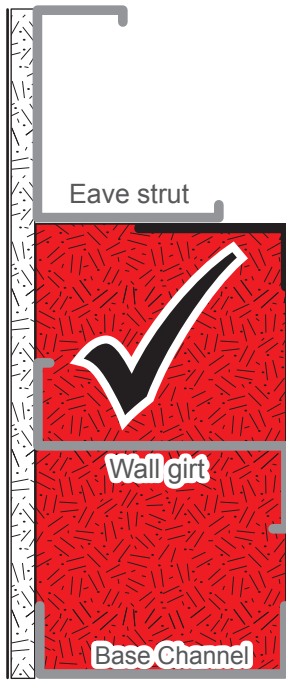
The insulation fills the cavity
