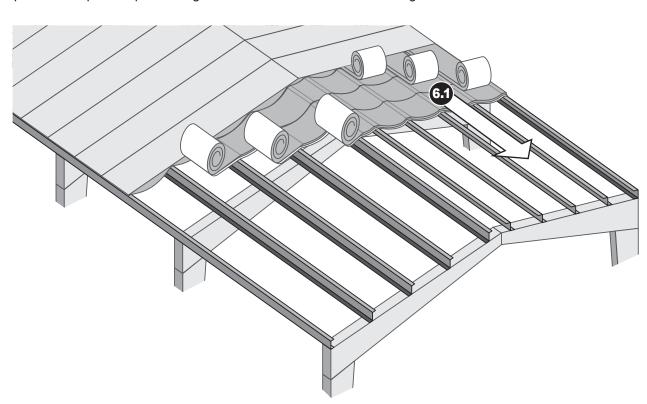
**6.2** Install roof panels. If thermal blocks are supplied they should be installed between the insulation and roof panels.
