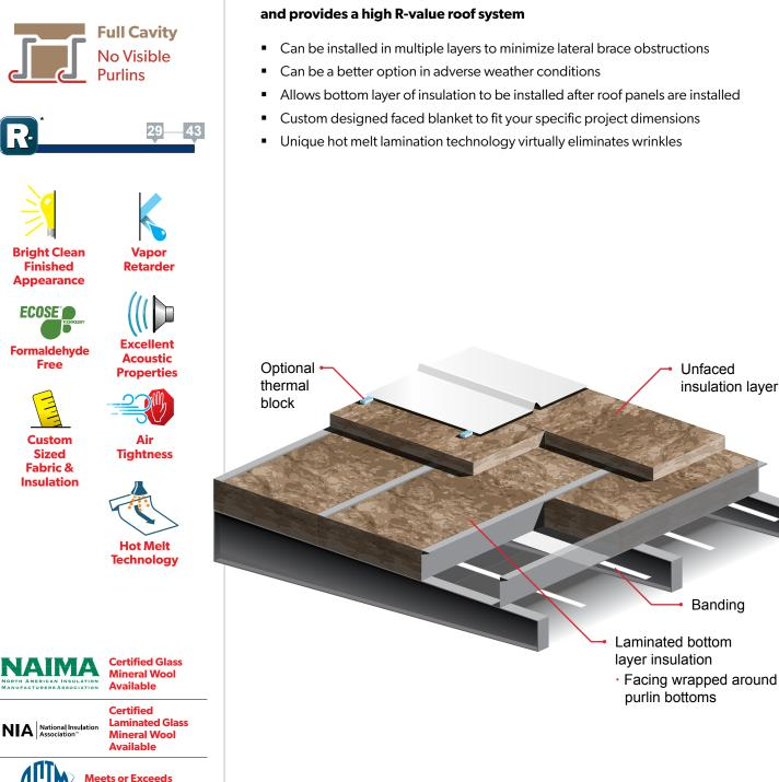
Banded roof insulation system that conceals purlins and fills cavity completely
