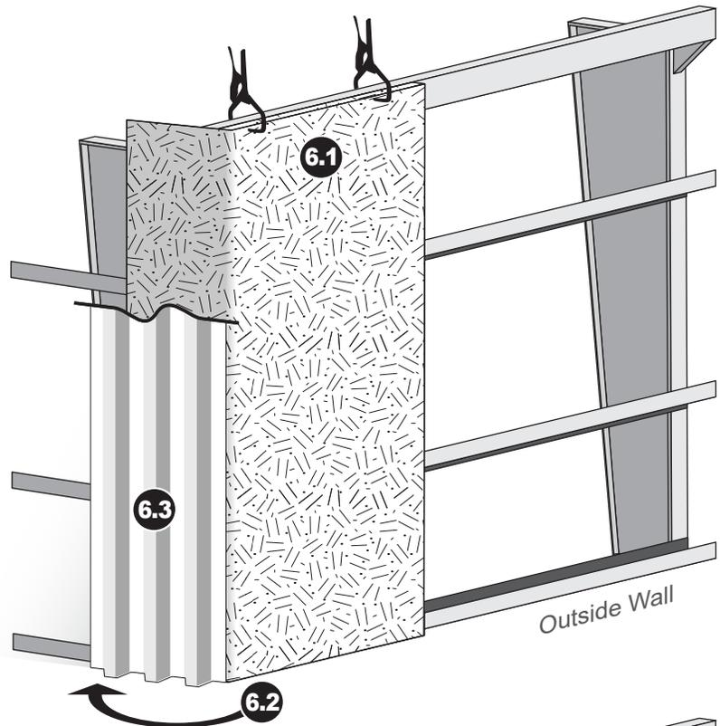
**6.4** Continue with insulation around the building and installing sheeting per the manufacturers' recommendations.
