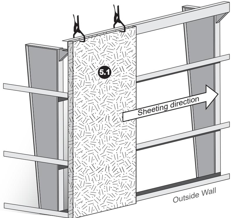
**5.2** Continue with insulation around the building and installing sheeting per the manufacturers' recommendation.
