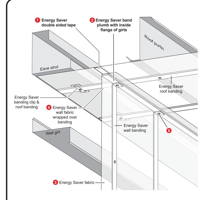
We recommend using a metal angle, not supplied by Silvercote, as the most durable connection (Technical Detail SIL800). While this angle may not be supplied as a standard part by many manufacturers it is typically available at an additional charge, or can be purchased locally.
