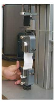
**TENSILE STRENGTH TESTING** - Silvercote conducts daily testing on actual production samples of welded Purlin Glide FP fabric to ensure your safety. Extensive drop testing has been performed to determine the actual failure point of the welded seam. Production samples must exhibit a seam strength of more than double the noted failure strength to meet our standards and be considered acceptable for use in a Purlin Glide FP system.
